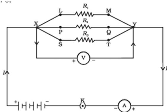
In the circuit diagram, suppose the resistors  $R_1$ ,  $R_2$  and  $R_3$  have the value  $5\ \Omega$ ,  $10\ \Omega$   $130\ \Omega$  respectively, which have been connected to a battery of  $12V$  then calculate -
